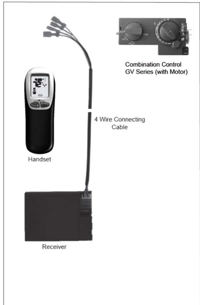
Figure 4: Wiring Diagram for OEM use only.
